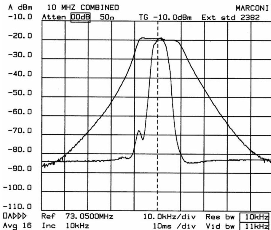
The result of the bandwidth improvement is the reduction of close in intermodulation from multiple signals. The IMD dynamic range will be improved up to 15 dB for signal spacings from 2 to 20 kHz. Also, the blocking dynamic range will be improved for close in signals.
