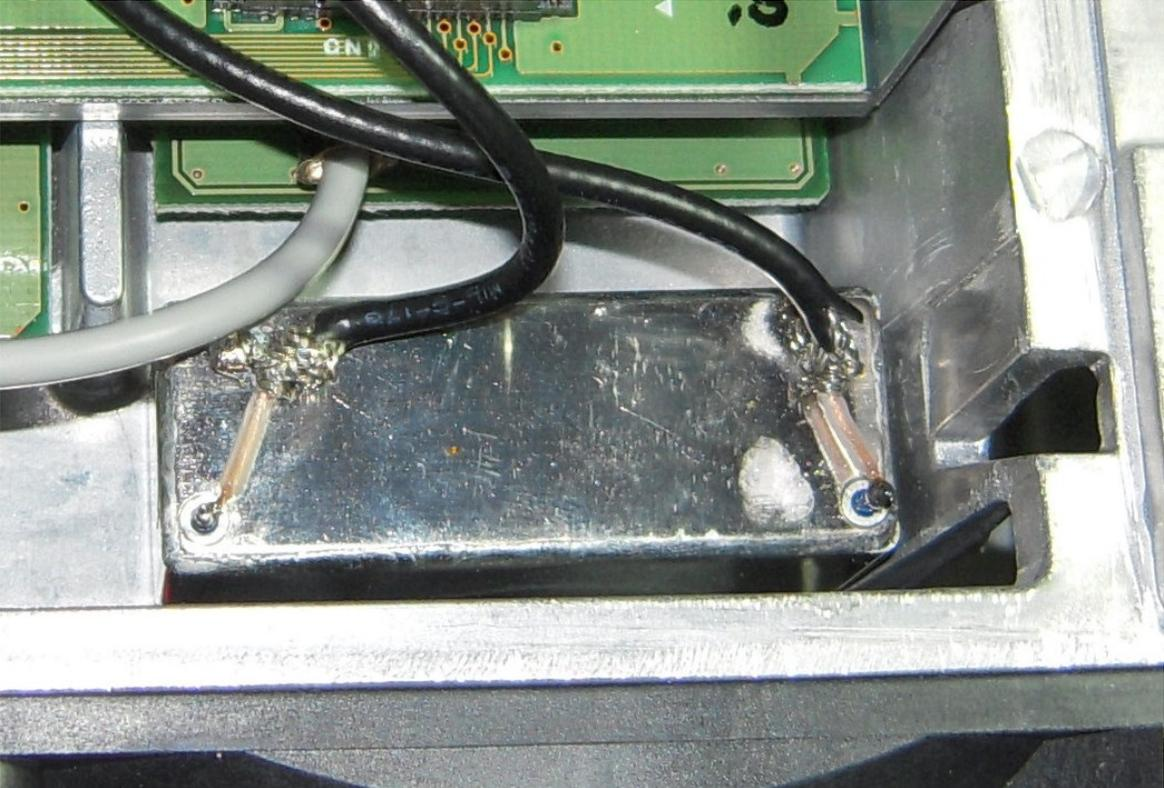
Figure 3. Cable connections to TX-RX1 PCB.
