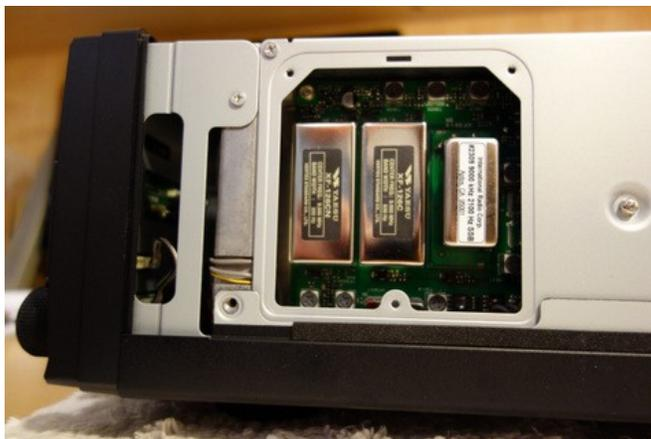
Figure 2. Inrad SSB filter installed
