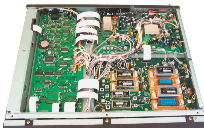
Figure 4—The roofing filter installed in an FT-1000MP Mark-V.
